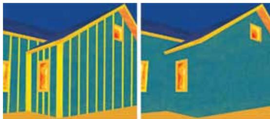
Heat loss due to thermal bridging in standard between-the-studs insulation
