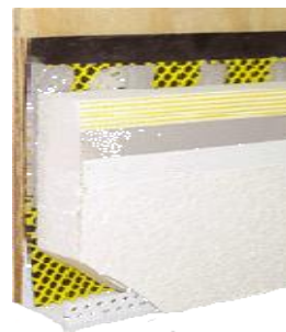
PB EIFS- Drainage mat mechanically fastened over building paper, EIFS applied with adhesives
