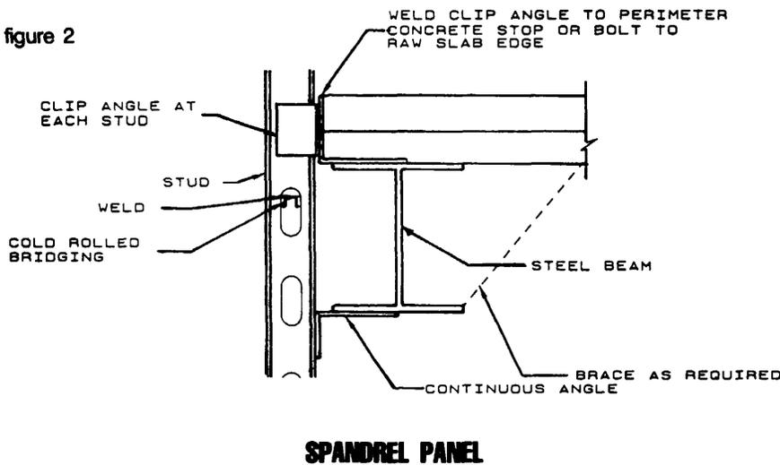
type panel previously described and illustrated in Figure 1. As can be seen in Figure 2, the spandrel panel is supported with an additional connection at approximately mid-span and slightly below mid-span with a connection to the spandrel beam, or it is connected near the bottom with a kicker, back to the floor or roof deck. This connection scheme leaves the spandrel panel with one or two cantilever overhangs, and normally a concentrated end load from the window it supports.
