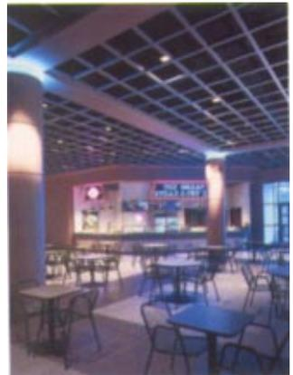
*The Cube 2 System utilizes the Tempra-4000 suspended grid system. Tempra is a conventional T-bar suspension system and is installed like any other grid system, except for a U-channel grid cover that is placed over the grid component to conceal the web of the T-bar, and to complete the illusion of a continuous ceiling plane.*
