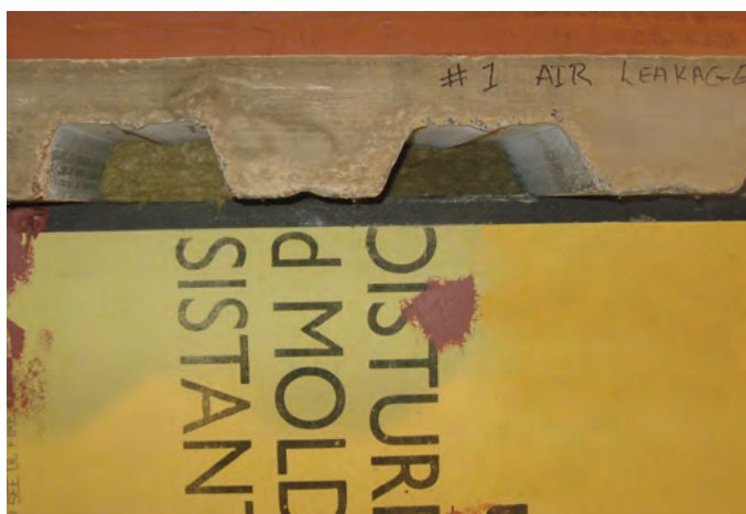
BlazeFrame deflection track & deck plugs in sound test
